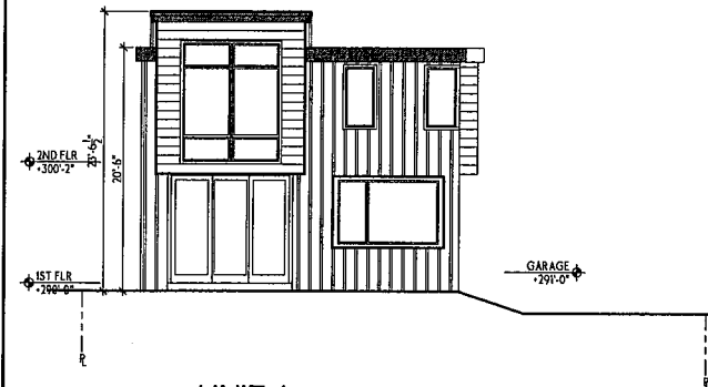
UNIT A REAR (SOUTH) ELEVATION 6 A3.0 1/8"=1'-0"
