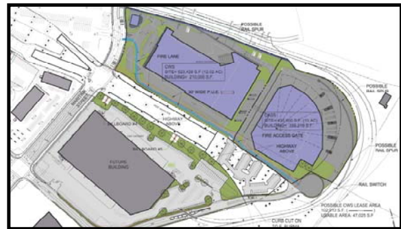
Site Plan for CASS & CWS at the City's portion of the former Oakland Army Base
