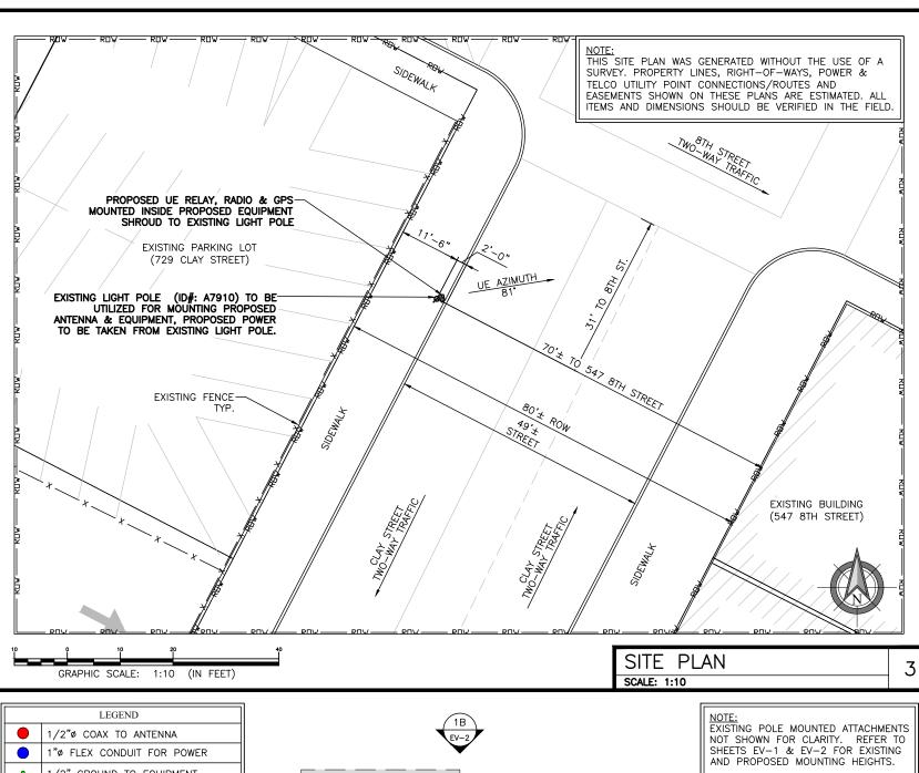
1/2"ø COAX TO ANTENNA 1"ø FLEX CONDUIT FOR POWER 1/2" GROUND TO EQUIPMENT
