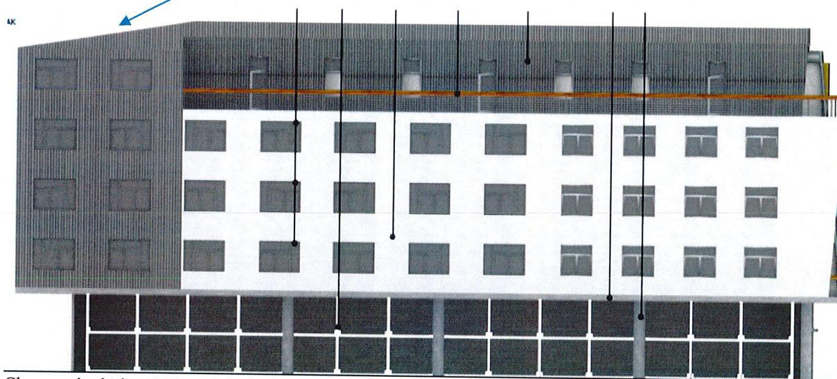
Changes include a 15' modulation created by removal of 7 units from the 5<sup>th</sup> floor which are replaced by a 25' roof deck and a 5' interior corridor. Building materials are also changed to reduce the amount of corrugated metal and substitute integral color medium white cement plaster. Prior West Elevation facing 532 30<sup>th</sup> St Condominiums
