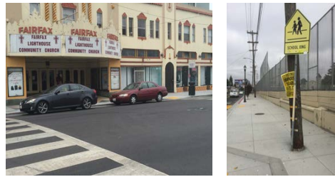
Exhibit C-14A: Parking Permitted In Intersection; School Crossing Sign Missing Crossing Directional Arrow
