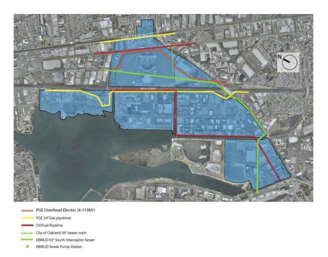
Figure 6.4: Utility Backbone Diagram
