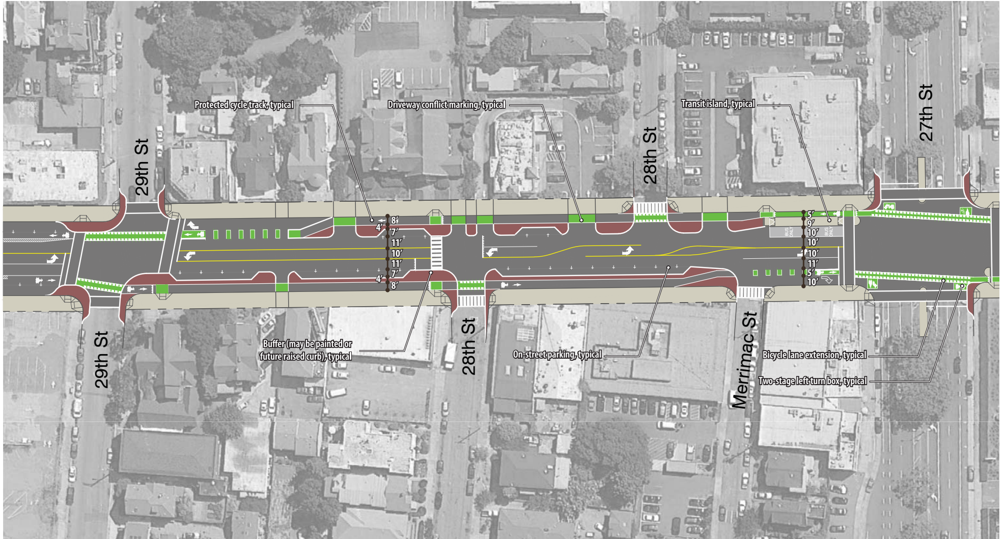
Figure A-8: Final Concept Plan Segment Drawings - 29th Street to 27th Street. The figure depicts a possible cycle track configuration.
