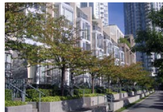
Primary residential entrances should incorporate projections, such as stoops, porches, recessed windows, and bay windows or balconies (DG-48).
