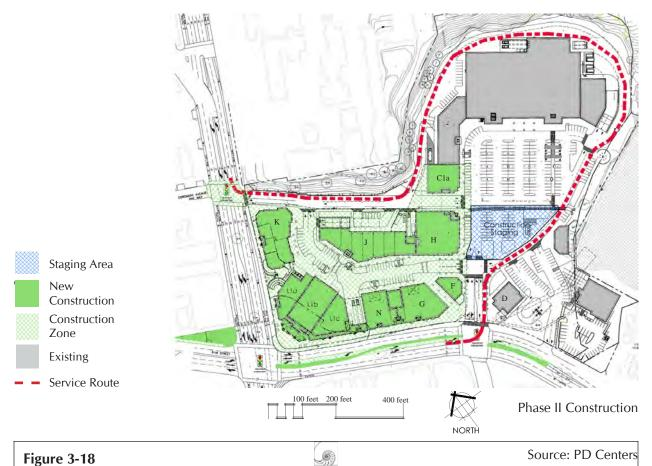
Figure 3-18 Project Phasing Plan, Phase II
