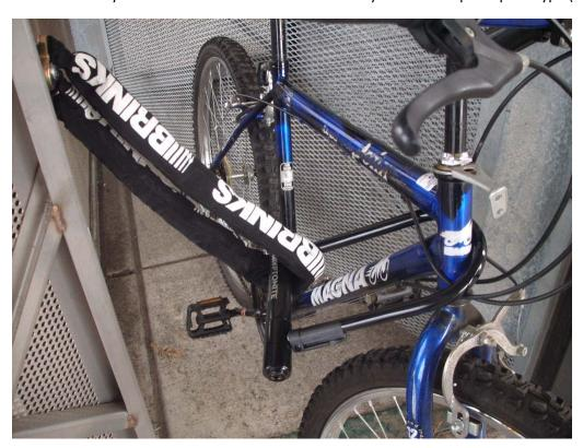
below and installed at the Berkeley Amtrak Station). The cost to install these is \$90/locker. The mechanism includes a 3' nylon-covered security chain (cannot be cut with bolt cutters), securely attached to the locker frame. The chain forms a loop which will reach the front of a bike parked in the locker. The
