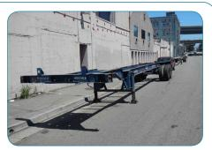
A bare chassis, one type of unattached trailer
