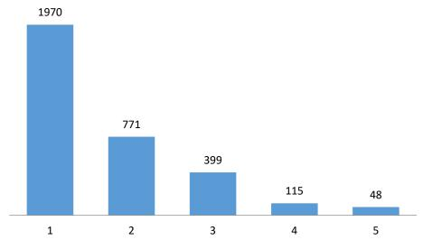
From a total of 3,330 pipe segments inspected, 1,970 segments were found to be in acceptable structural condition (Grade 1), 771 segments were found to be in minimal collapse risk condition (Grade 2), 399 segments were in collapse unlikely in near future condition (Grade 3), 115 segments were found to be in collapse likely in foreseeable future condition (Grade 4); and 48 segments were found to be in danger of imminent collapse (Grade 5).
