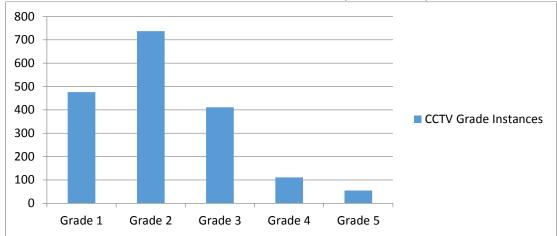
From a total of 1,790 pipe segments inspected, 476 segments were found to be in acceptable structural condition (Grade 1), 737 segments were found to be in minimal collapse risk condition (Grade 2), 411 segments were in
