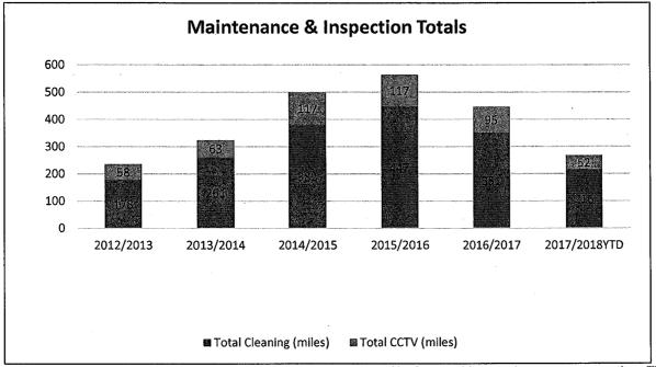
Figure 2 - Approximately 60% of total annual cleaning, and 85% of annual inspections, are preventive. The remaining work is done in reaction to system emergencies and/or imminent failure that could result in overflows.
