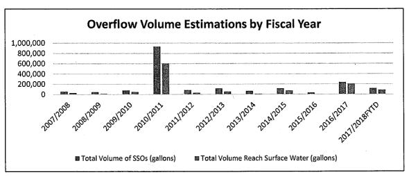
Figure 4 - Sewer overflow volumes are calculated by using visual observation and estimated duration. Geometric analysis may be used when an overflow has been completely contained. All volume calculations are best estimates only. Efforts are made to ensure that volume calculations are documented and defensible.
