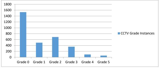
From a total of 3,224 pipe segments inspected, 1,534 segments were found to be in excellent structural condition (Grade 0), 495 segments were found to be in acceptable structural condition (Grade 1), 688 segments
