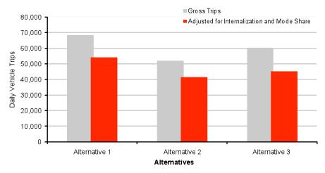
Figure 3.1: Daily Vehicle Trip Generation Comparison
