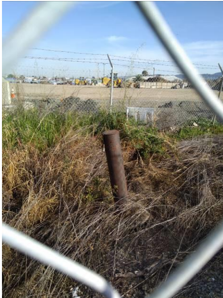
Photo #13 View of a monitoring well, located on the northern portion of the site.
