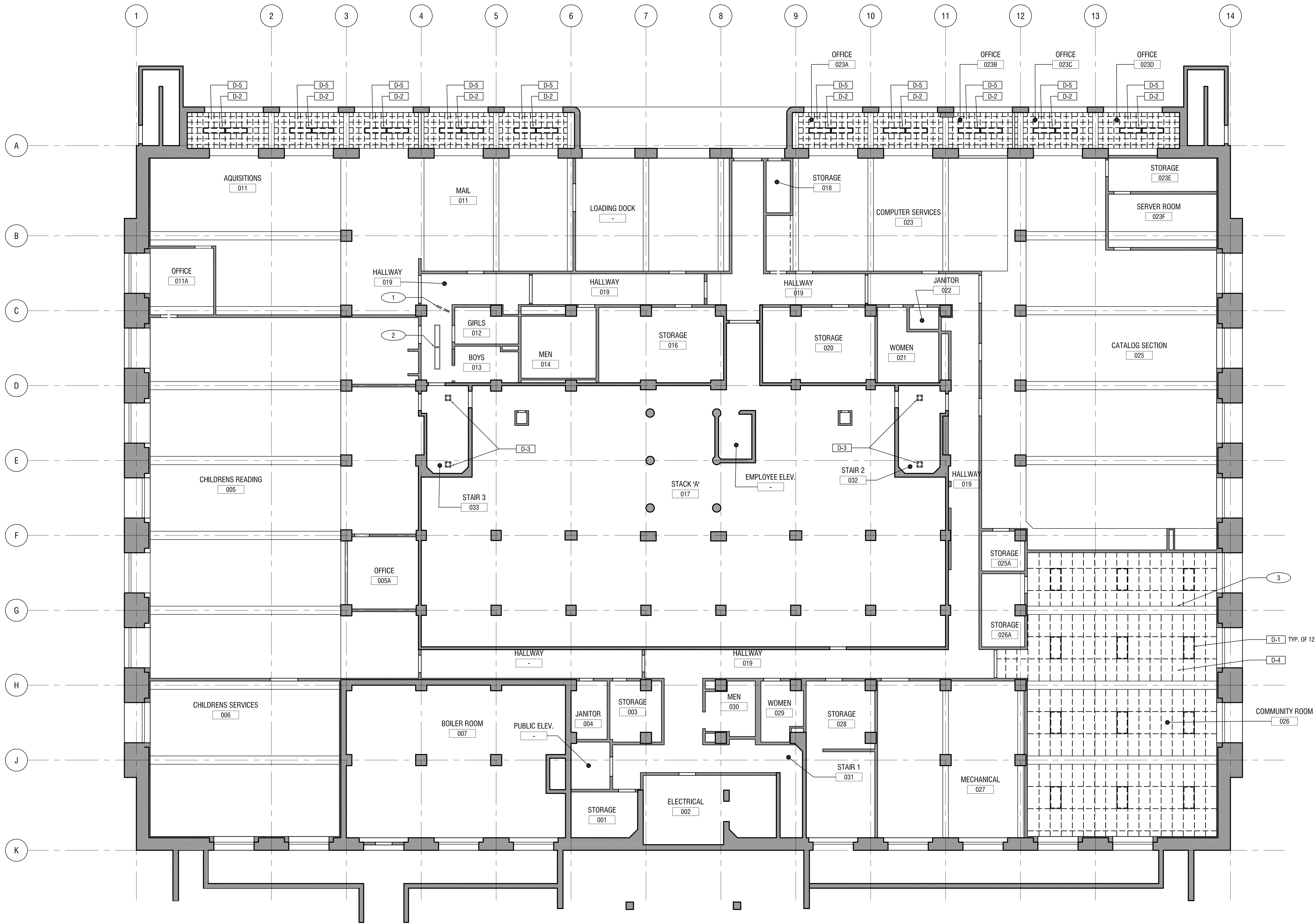
1 LEVEL 1 - GROUND FLOOR DEMOLITION REFLECTED CEILING PLAN SCALE: 1/8"=1'-0"
