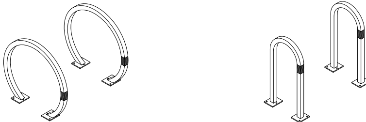
RACK TYPES: Flange-mounted, square-tube, galvanized steel; U- and circular-styles (shown w/ 4" white reflective tape adhered to the travel lane side of the rack footer).
