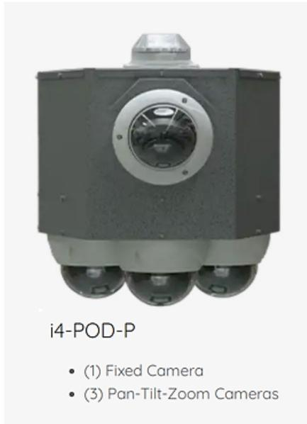
The **Portable Observation Device**, or POD, is an all-in-one, portable surveillance system. The i4POD-P has four (4) cameras and includes a digital video recorder, a cellular router and a wifi transmitter – all housed in an easy to move and mount enclosure. The POD is plug and play; the City needs only to supply 110v power to activate system.
