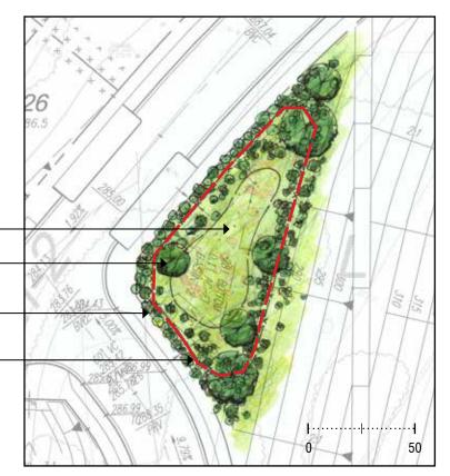
Figure 29 - Typical Detention Basin Plan
