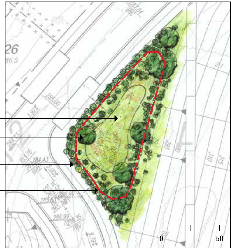
Figure 29 - Typical Detention Basin Plan
