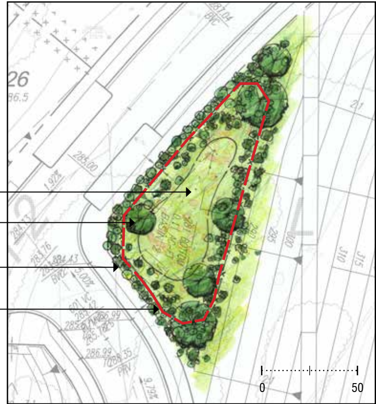
Figure 29 - Typical Detention Basin Plan
