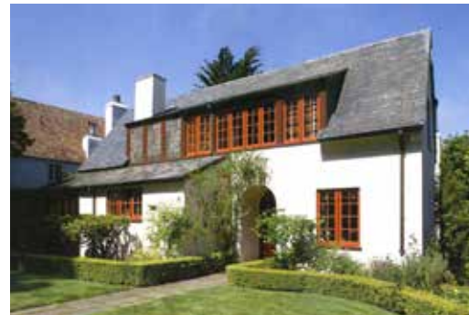
12/12 steeper pitch roof with dormers
