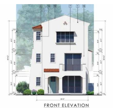
3 BOARD & BATT SIDING 4 SHINGLE SIXING 5 VINYL WINDOW 6 SHUTTERS AT ENHANCED ELEVATION 7 WROUGHT IRON RAILING B STANDING SEAM METAL ROOF 9 FLAT CONCRETE TILE ROOF 10 S-TILE ROOF 11 GARAGE DOOR 12 STANDING SEAM METAL CANOPY 5HUTTERS AT ENHANCE CONDITION FACING STREET 14 WINDOW WOOD TRIM 15 STONE VENEER 16 EXTERIOR LIGHTING 17 UTILITY LOCATION / ROOM TO BE DERTERMINED 18 AC LOCATION 19 PRIVACY FENCE AT END UNIT **ELEVATION KEY NOTES**
