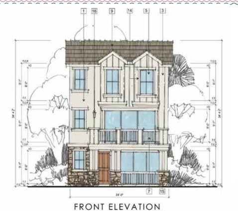
1 STUCCO 2 HORIZONTAL SIDING 3 BOARD & BATT SIDING 6 SHUTTERS AT ENHANCED ELEVATION 7 WROUGHT IRON RAILING 8 STANDING SEAM METAL ROOF 9 FLAT CONCRETE TILE ROOF 10 S-TILE ROOF 11 GARAGE DOOR 12 STANDING SEAM METAL CANOPY 13 JULIET BALCONY 14 WINDOW WOOD TRIM 15 STONE VENEER 16 EXTERIOR LIGHTING 17 UTILITY LOCATION / ROOM TO BE DERTERMINED 18 AC LOCATION 19 PRIVACY FENCE AT END UNIT 20 TILE ACCENT 21 DECORATIVE WOOD RAIL **ELEVATION KEY NOTES** PARCEL A
