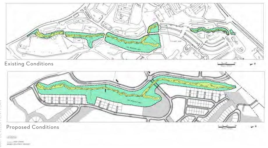
Figure 20 - Existing Rifle Range Creek Corridor and Proposed Restoration Area
