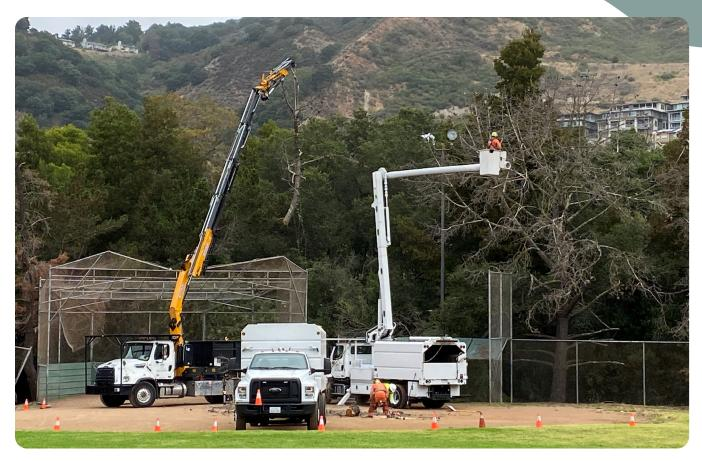
▲ The Parks & Tree Division uses a variety of specialized vehicles to perform tree work throughout Oakland. Pictured: crane (left) picks up dead tree stem for removal and disposal, chip truck (middle) collects wood chip debris from a chipper attached to it on the rear (not visible in photo), large aerial (right) allows tree trimmers to safely access trees for pruning and removal work.
