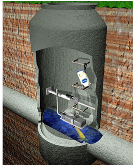
Figure 14. Typical Flo-Dar Flow Meter Installation
