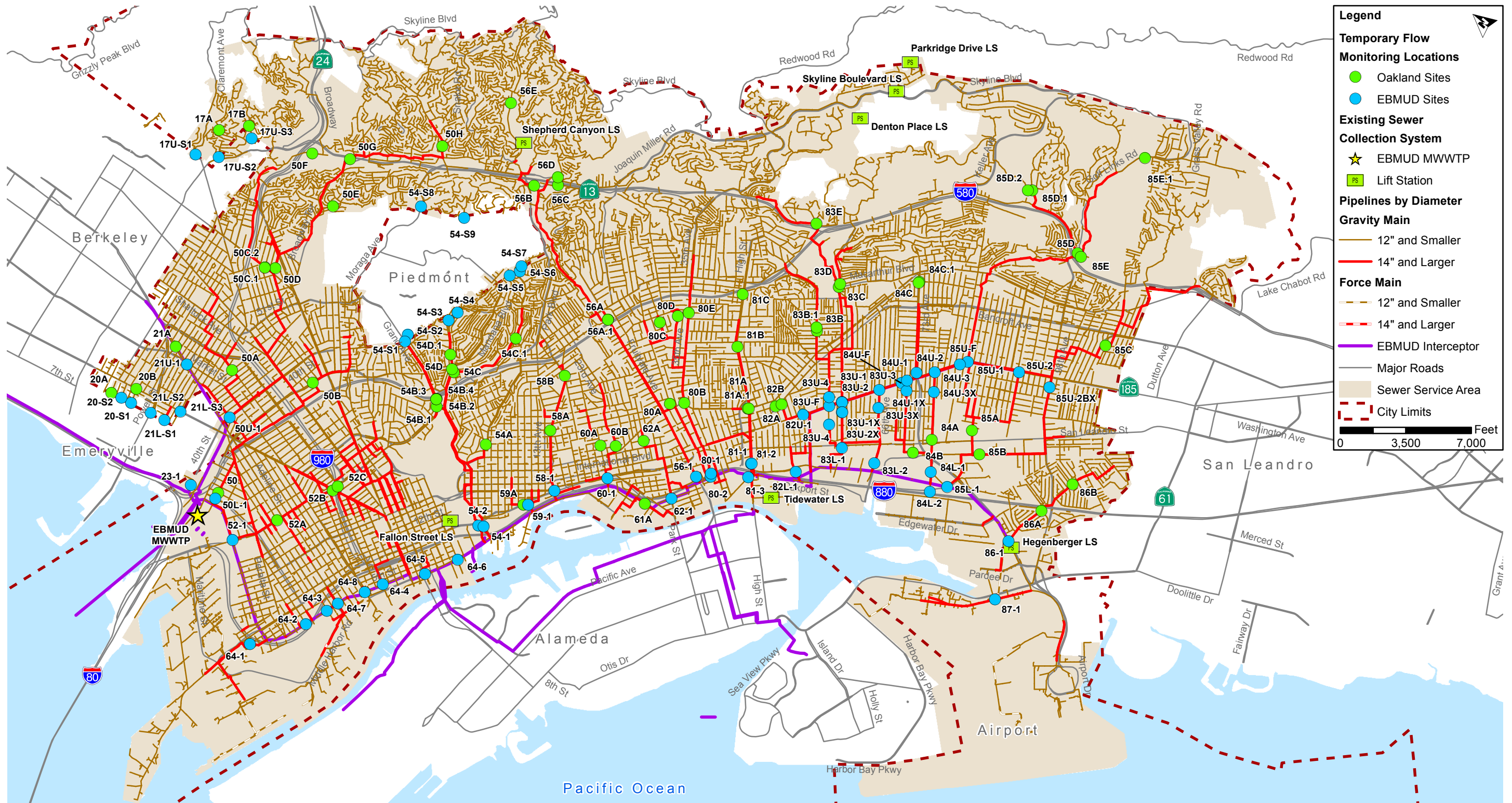
Figure 3.4 TEMPORARY FLOW MONITORING LOCATIONS SEWER SYSTEM HYDRAULIC MODELING AND CAPACITY ANALYSIS REPORT CITY OF OAKLAND
