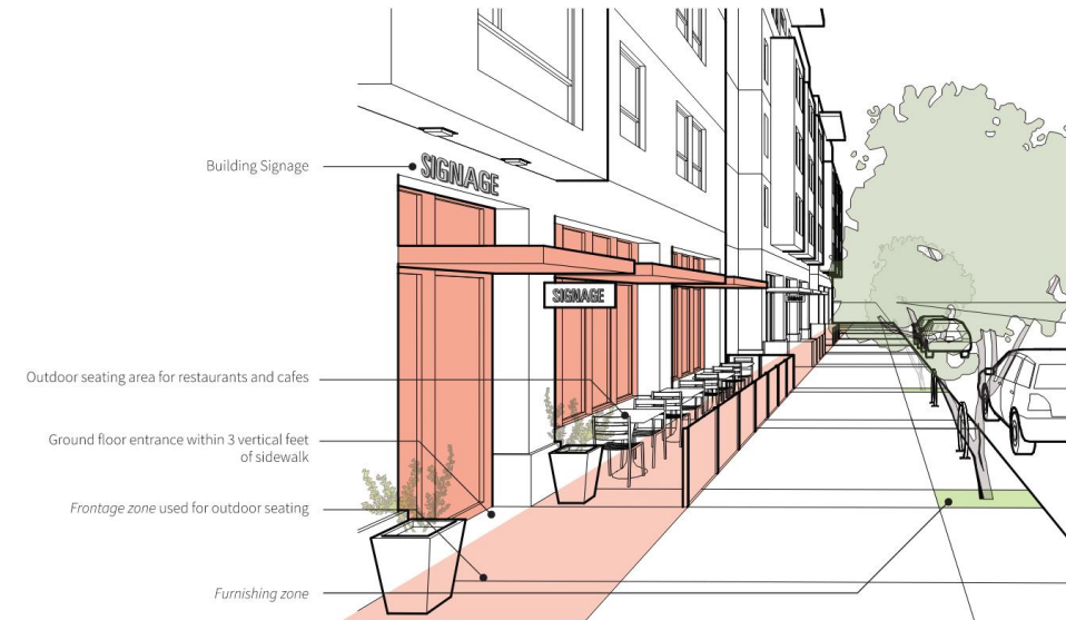
Fig. 4.4 Provide a setback for commercial frontage along primary streets to allow for transitions, frontage zones for outdoor seating, and future sidewalk widening.
