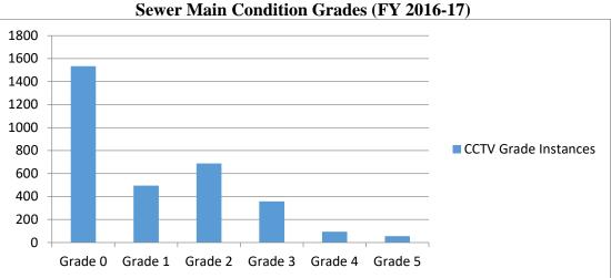
Figure 4-1 Sewer Main Condition Grades (FY 2016-17)
