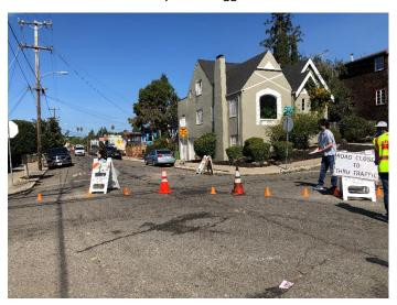
Figure 6. Diagonal diverter made with chalk and cones
