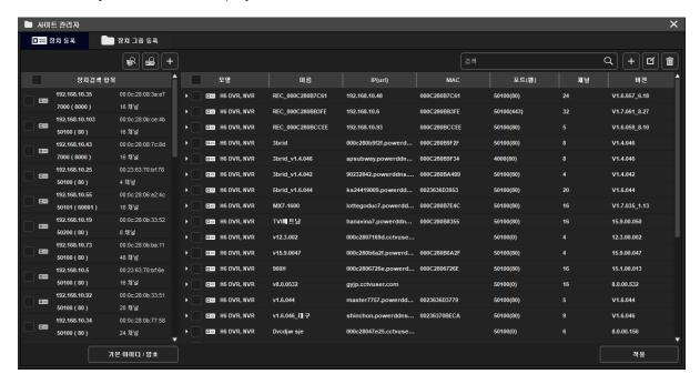
Please select device at below to register device to NETUS and Press button, then selected device is supposed to be registered to right side tab.
