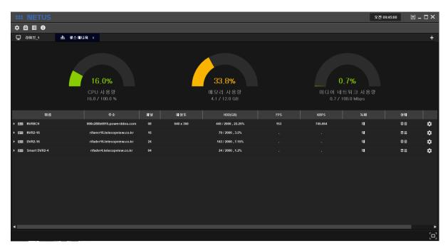
You can see the name, address, channels, resolution, HDD status, FPS, KBPS, recording, network status and detailed info of each registered device.
