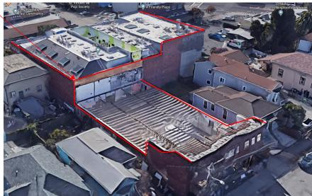
6.Provide Structural Steel bracing that run the full length of the East and West terra cotta walls and attach directly, at the inside face of the wall, in order to stabilize and seismically retrofit in a liquefication zone.
