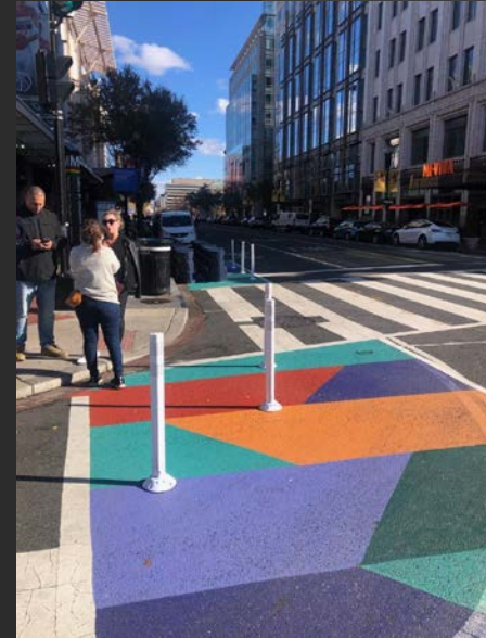
Washington D.C. Intersection corner has flexposts that prevent sharp turns
