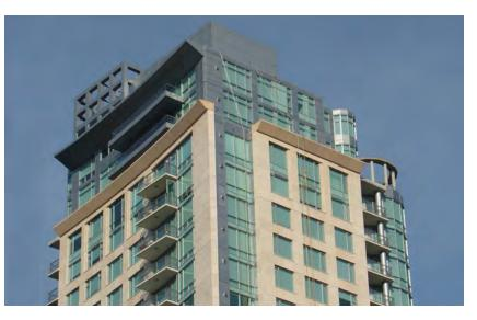
The topmost floors of towers should be architecturally differentiated through the use of stepbacks, changes in material, building shape, etc.
