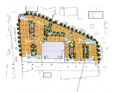
Revised 2015 FPUD Site Plan for Phase IIA that affect Phase IIB shows changes in the parking garage affecting both properties. The location of the parking is still along the BART tracks but it is incorporated into the 4-story housing development. Open space is moved to the interior and the future shared 'Paseo" between Phase IIA and Phase IIB is identified. This is an enlargement of half of the original PUD site plan
