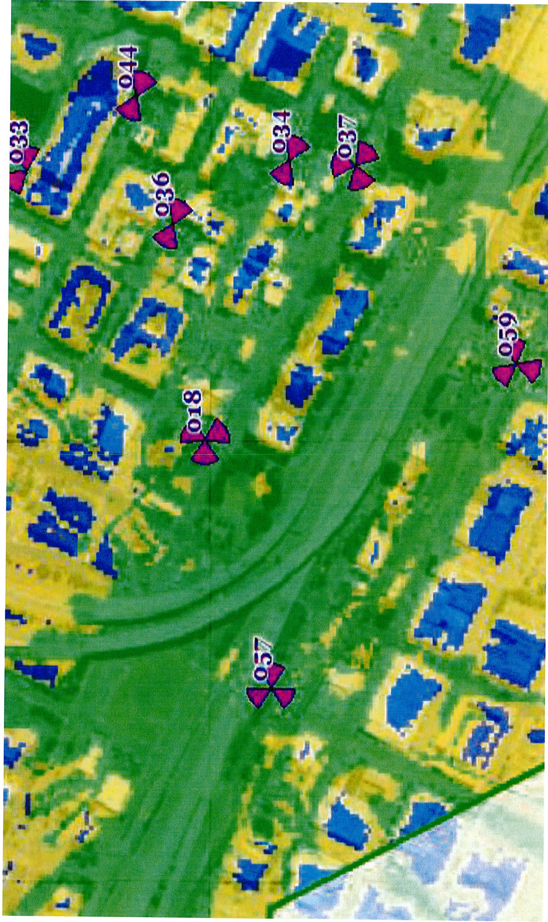
This propagation map depicts the ExteNet proposed Node 00057A in relation to surrounding proposed ExteNet small cell nodes.
