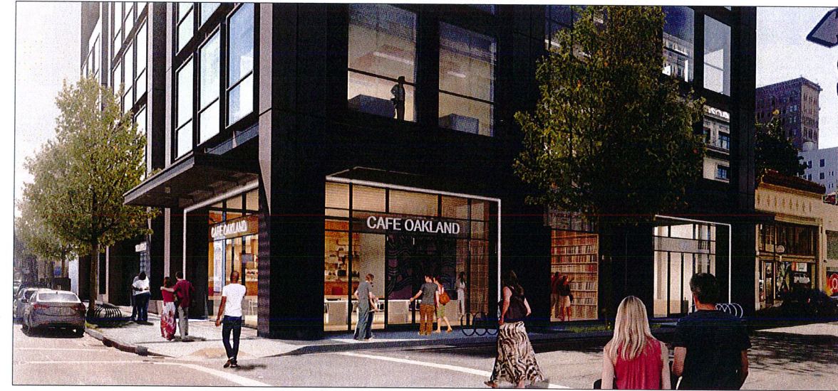
METAL SIGNAGE ATTACHED TO AN OBSCURED GLASS BACKING PANEL SIGNAGE ILLUMINATED BY DOWNLIGHTS IN THE CANOPY
