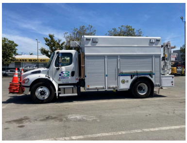
Large Valve Truck
