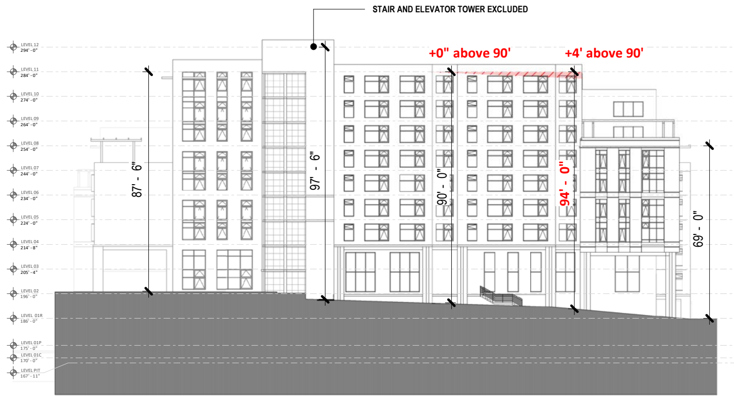
ELEVATION - BUILDING A EAST 1" = 40'-0"
