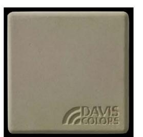
3. CIP Concrete Paving - Finish 3 Oakland City Standard Mix: 520-C-2500 with a pound or pint of "Lamp Black" per cubic yard Finish: Top-Cast, Acid Etch Sawcut control joints
