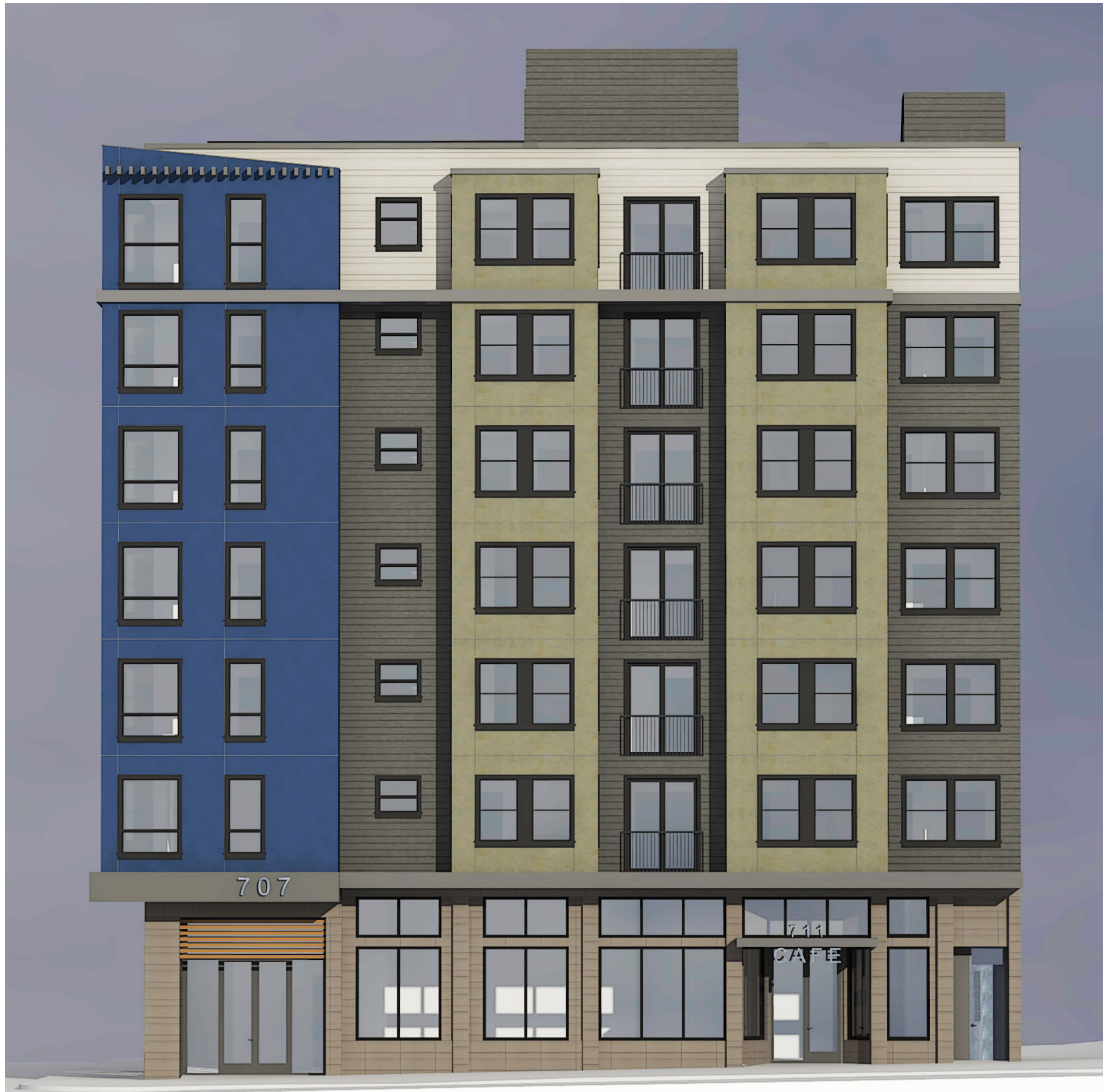
BLUE SHADE COLOR AT CORNER BAY - 3-COAT EXTERIOR STUCCO w/ SMOOTH FINISH
