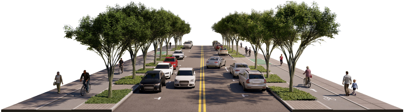
Figure AP/B-5: 3rd Street Extension, Option 1 (with elevated bike lane)
