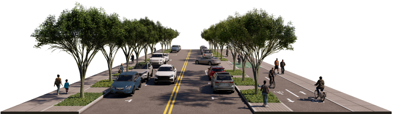
Figure AP/B-7: 3rd Street Extension, Option 3 (with elevated cycle track)
