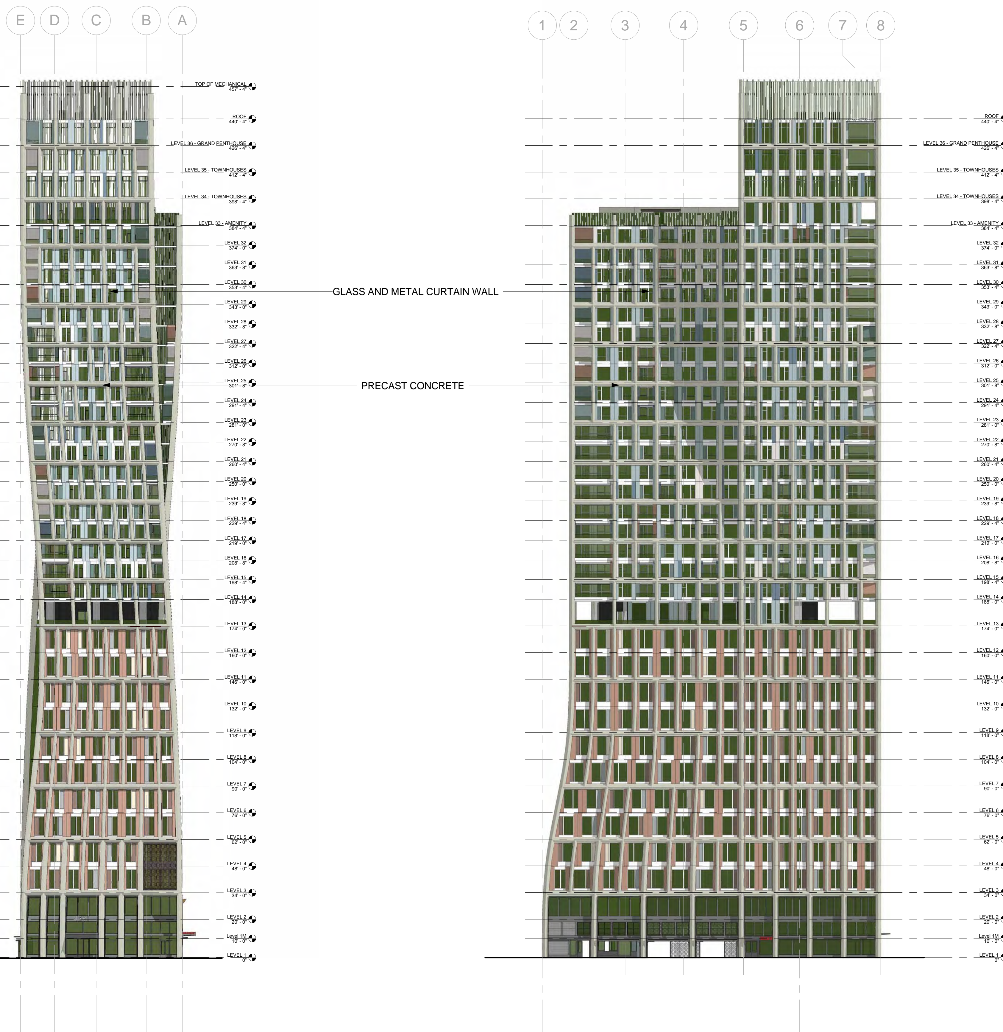
② SOUTH ELEVATION Copy 1 1" = 30'-0"
