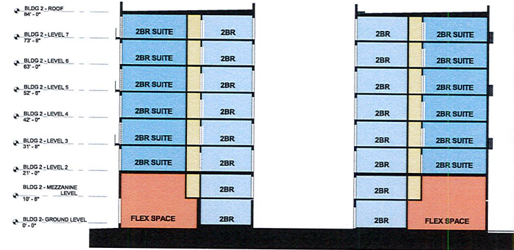
3) BUILDING 2 - SECTION THROUGH COURT 1/16" = 1'-0"
