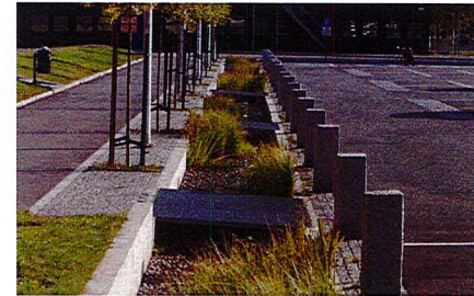
BIORETENTION BASIN w/ METAL GRATE
