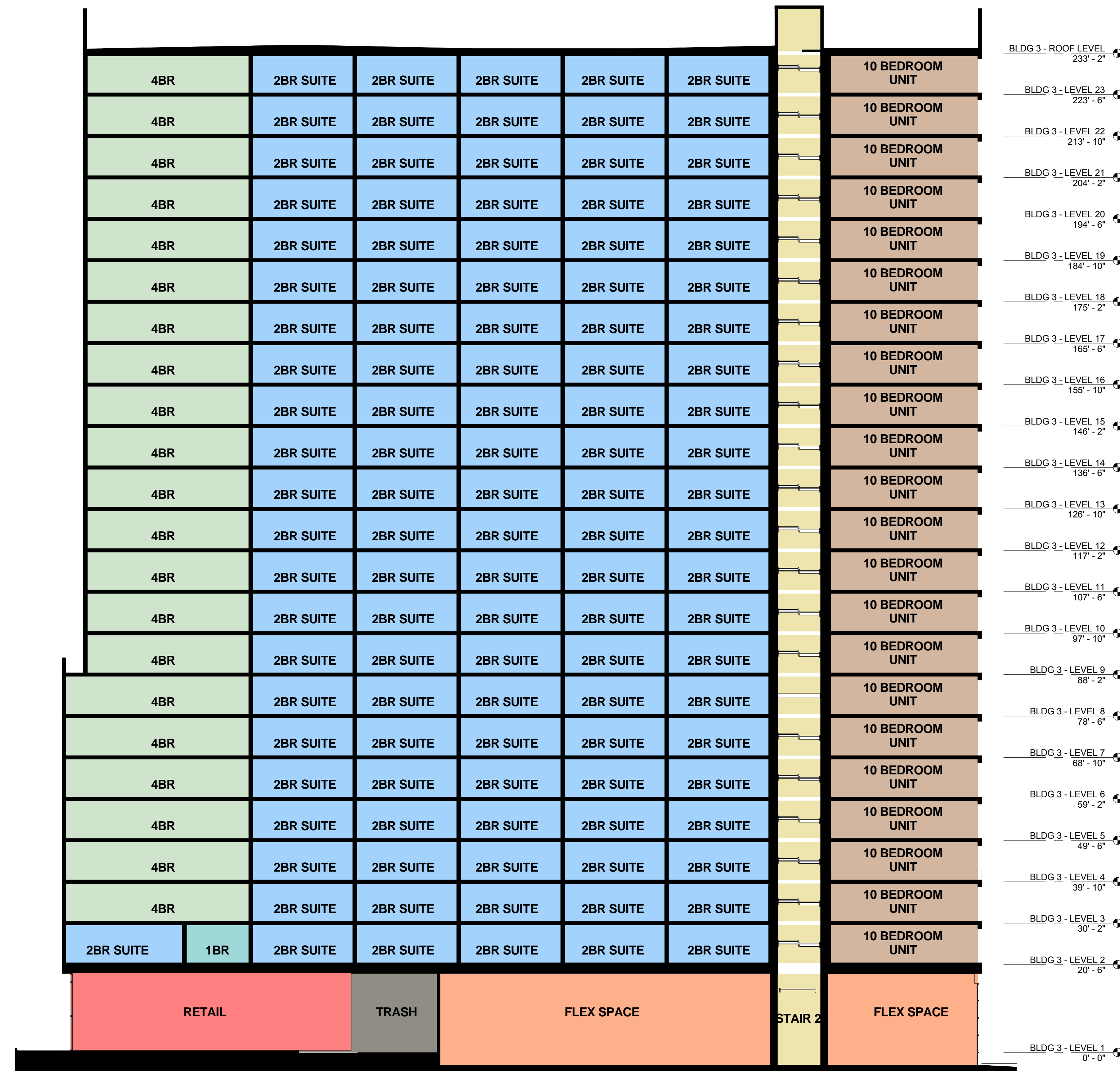
2 BUILDING 3 - SECTION THROUGH COMMERCIAL & CORRIDOR @ UNITS 1/16" = 1'-0"
