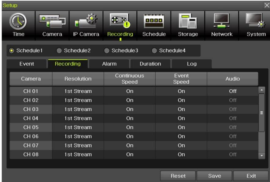
[Figure 3-23. Recording Setup Window]
