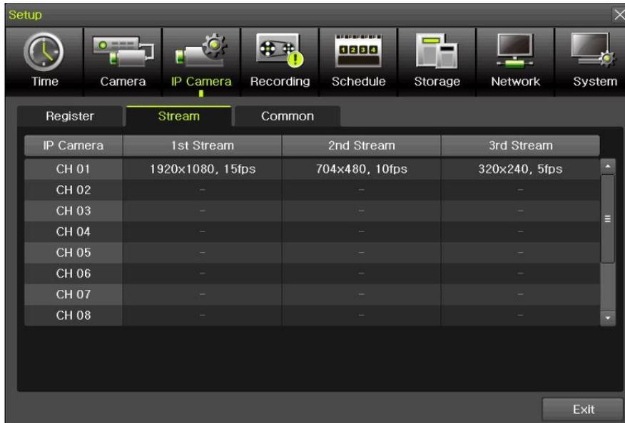
[Figure 3-19. IP Camera Stream Setup]
