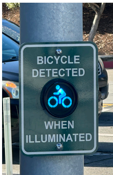
2. The detector light illuminates when a bicyclist waits at the intersection.
