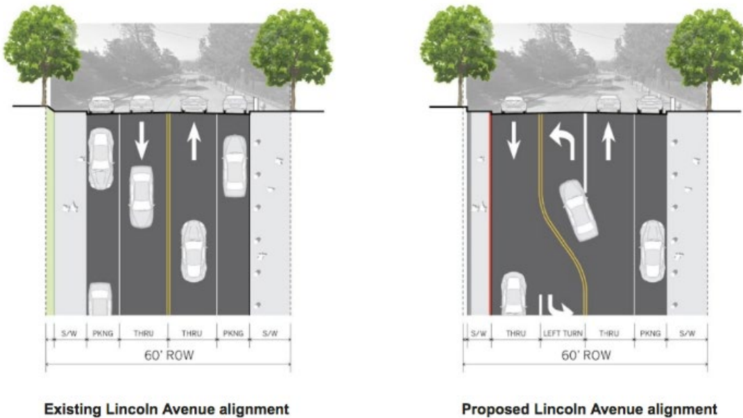
Figure 5 Existing & Proposed Typical Lincoln Avenue Lane Alignments
