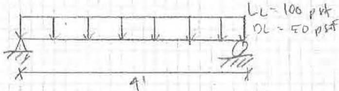
$$1.2 DL + 1.6 LL = (50 \text{ psf}) \times 4' + 1.6(100 \text{ psf}) = 220 \text{ psf}$$
