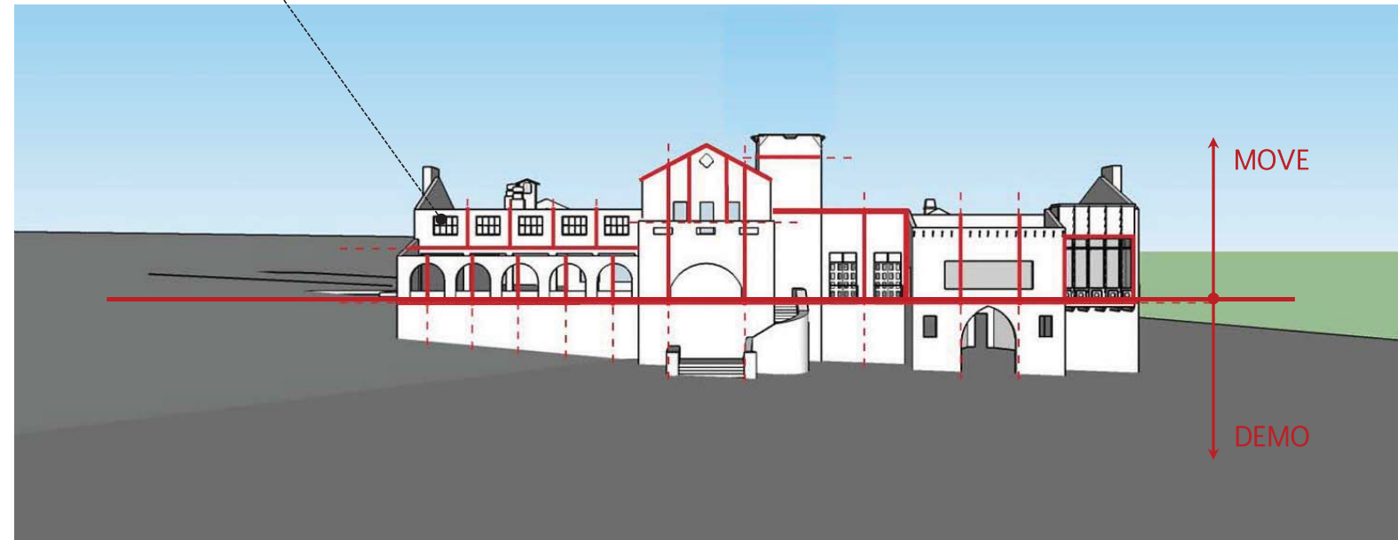
11 CUT AND SALVAGE WALLS
