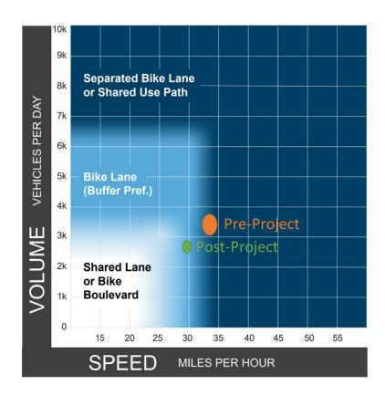
The project made West St a more suitable bikeway connection by reducing vehicle volumes and speeds.
