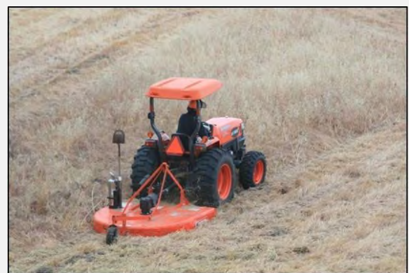
Exhibit 6. Mower attachment on a tractor.
