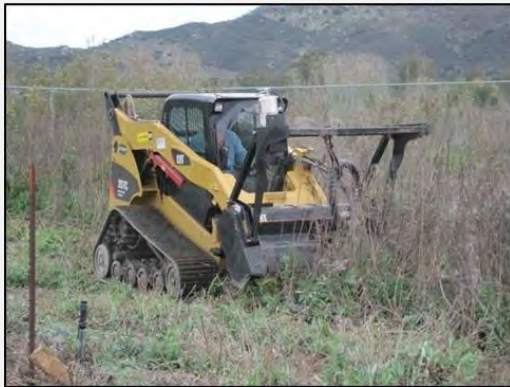
Exhibit 8. Masticator attachment on a bobcat.
