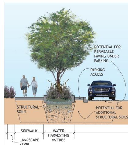
► *Figure 3.11.c: Structural soils provide a load bearing medium that also has the ability to maintain necessary voids for root growth.*
